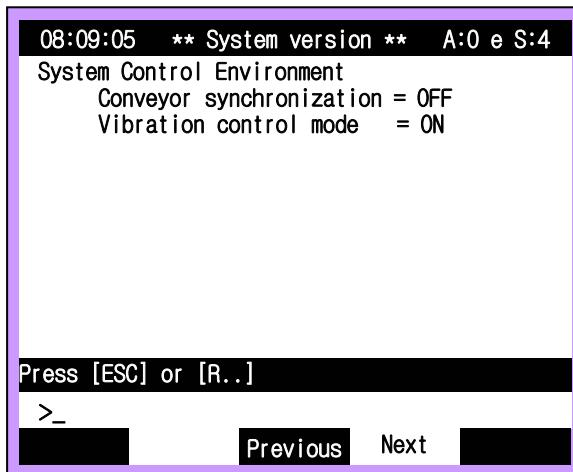
Since the vibration controller controls the robot based on robot dynamics, load data of tool is necessary to improve control performance.
