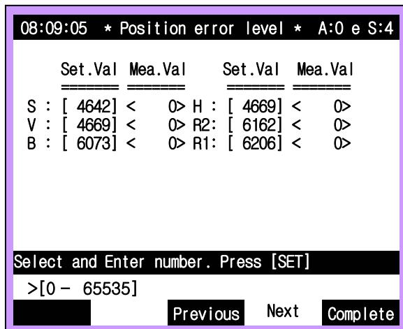
Set a deviation value to detect axis deviation error 『E0117 ○Ax) Too large position drift』 when unusual moves are found in robot performance.
