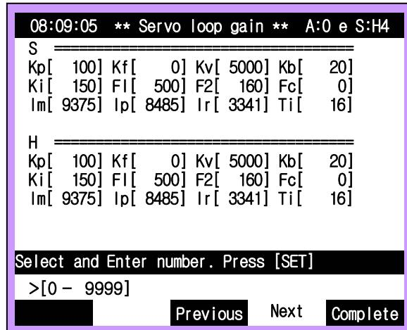
Set each gain of the servo controller. If servo loop gain is changed, this immediately affects the servo controller. Therefore, it is safe to change the gain when motor is off.
