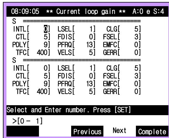
Hi4a controller is embodied with full digital servo, and motor current control is also digital type. Changed current loop gain is also run after the controller power is turned off and then on again.
